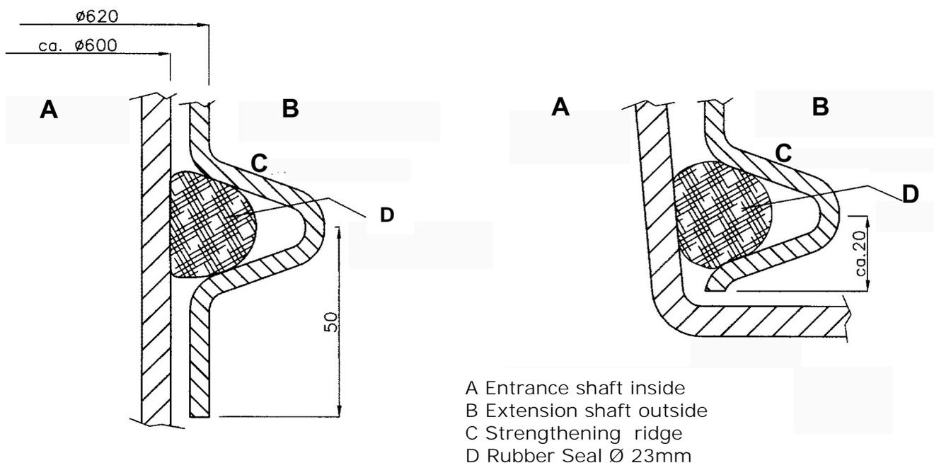
Note: For products with short entrance shaft, such as the Monolith, ET / Tubus or F-Line tank, the extension shaft has to be shortened about approx. 30mm.
